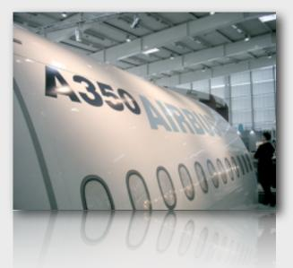
The A350's fuselage and cabin physical mock-up is being assembled at Airbus's Hamburg plant, with the front fuselage so far having been constructed. "In the coming months the whole fuselage will be built - we have already used it a lot last year for testing design, assembly processes, tools and jigs," adds Evrard.
